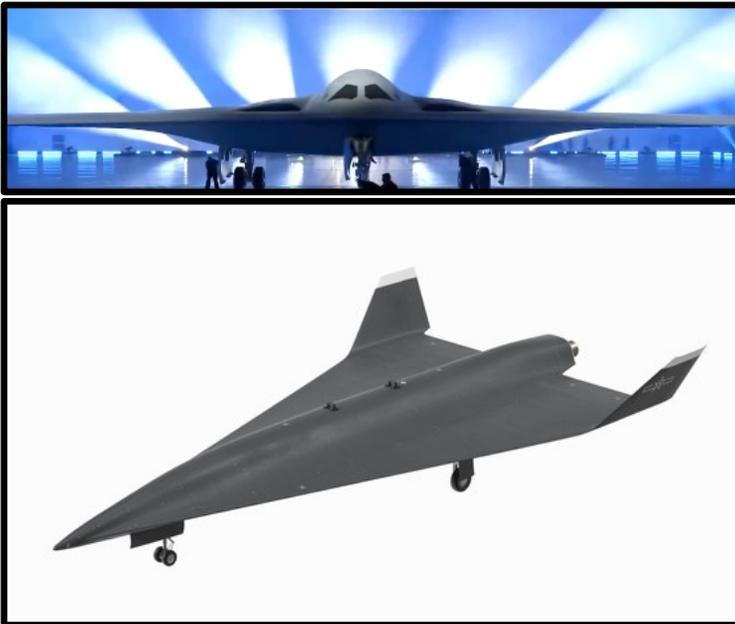
Figure 1. Top: The B-21 Raider stealth aircraft, showing the thin cross-sectional area and aerodynamic design to reduce air friction and shock waves. Bottom: China's WZ 8 Hypersonic Surveillance Drone. Thin frontal cross-sections are vital to reduce air friction and shocks.
